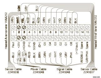
Figure 1. WAC151 Standard Wiring for WAA252 and WAV252
