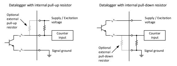
Figure 2: P2546D-OPR connection using an internal pull-up (left) or pull-down (right) resistor.
