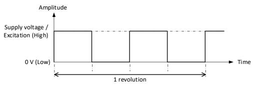
Figure 3: Datalogger counter input waveform.
