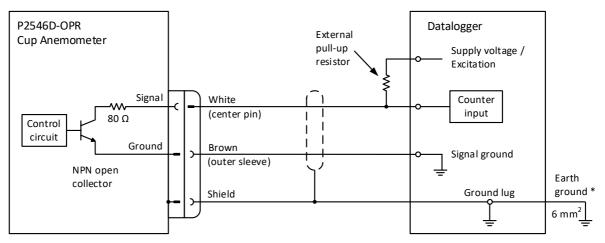
\* Connect the datalogger's ground lug to earth ground. Connect the ground lug to the nearest point at a met. tower or turbine structure, and trim the wire to the shortest possible length. Maintain the integrity and continuity of the shield connection in all intermediate junction boxes used.
