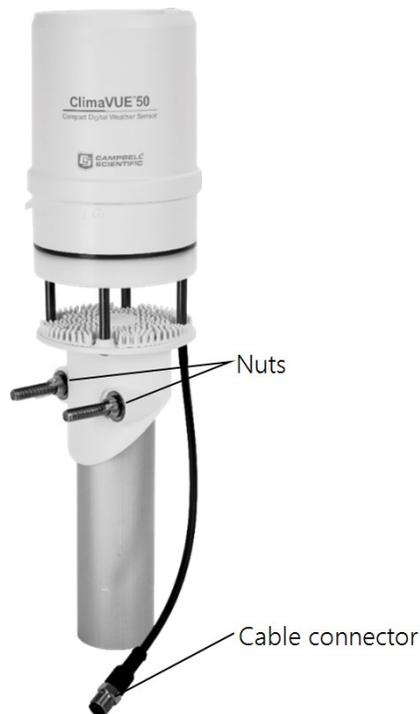
*FIGURE 7-5. ClimaVUE 50 with connector cable*
