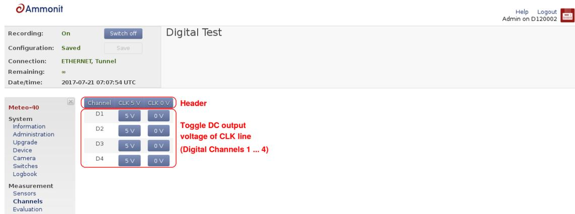
Figure 11.1: Configuration Menu for CLK-Line Test in Meteo-40.
