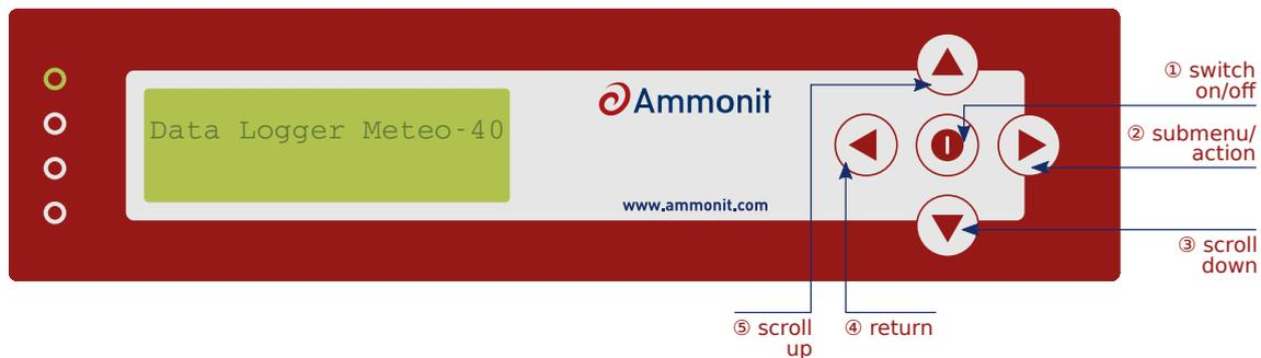
Figure 9.1: Use of the Meteo-40 buttons
