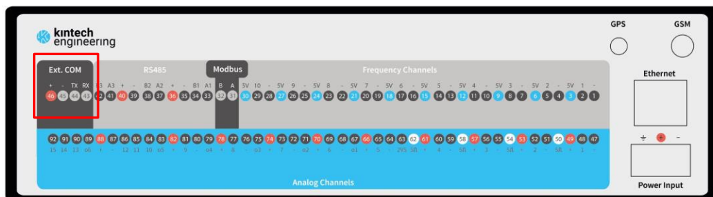
Fig. 70. Direct COM terminals: 44 and 43
