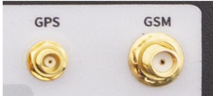
Fig. 10. GPS and GSM antenna connectors
