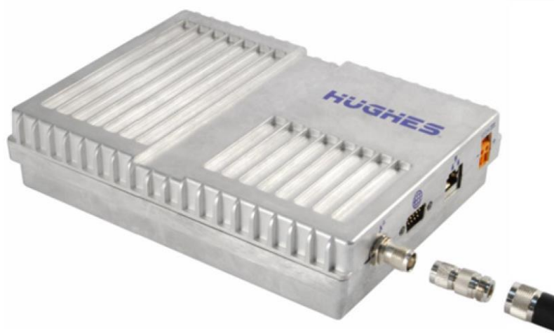
Fig. 68. BGAN satellite modem (logger side)
