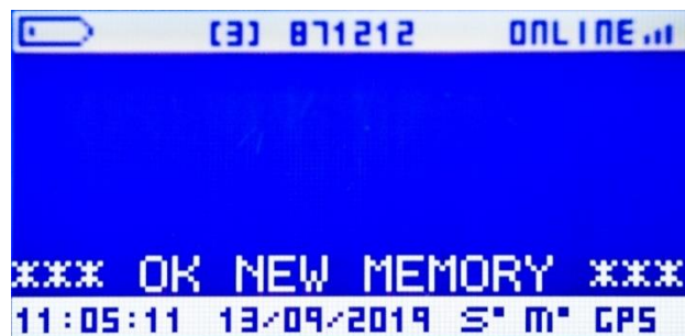
Fig. 59. Display: new storage cycle screen
