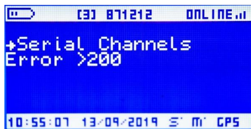
Fig. 39. STATUS screen: Serial Channels
