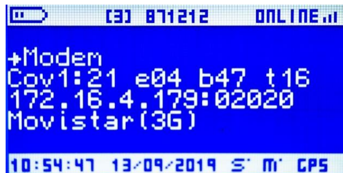
Fig. 74. Logger display: status > modem > e04 (logger online)
