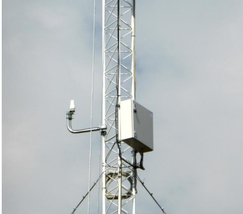
Fig. 65. Iridium antenna for satellite connection
