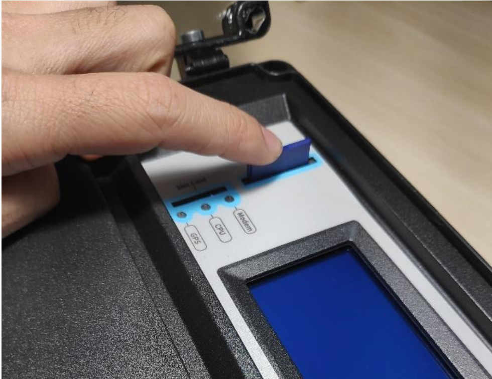
Fig. 56. How to take out the SD card
