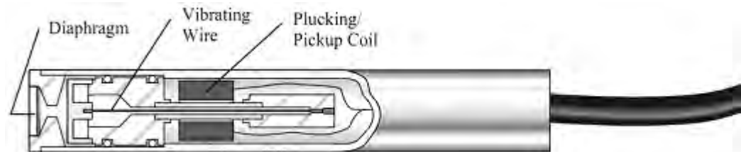
Figure 96. Vibrating-Wire Sensor
