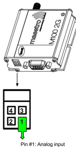
1. Connect an external analog voltage of maximum 5V.
