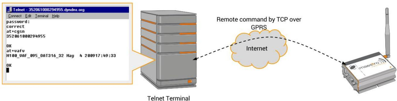
Figure 7.1.1: Example of TCP Terminal using Telnet
