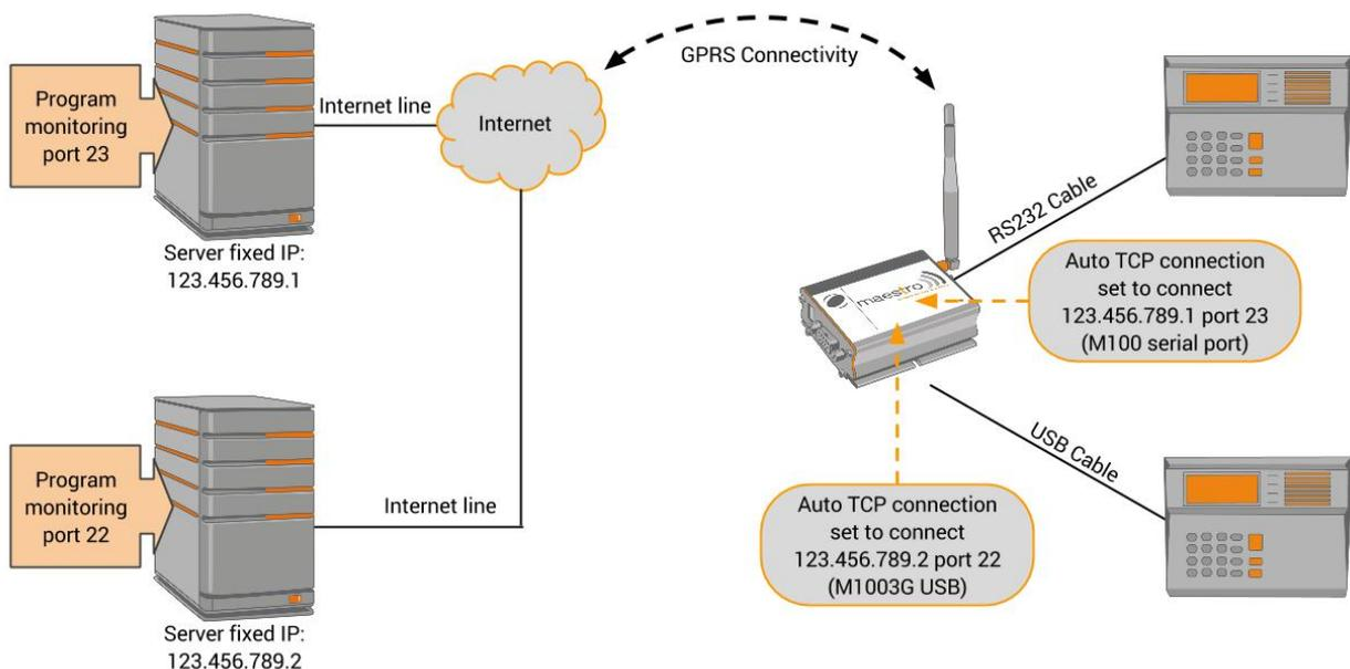
Figure 3.0.2: Example of Automatic Connection(s) over GPRS
