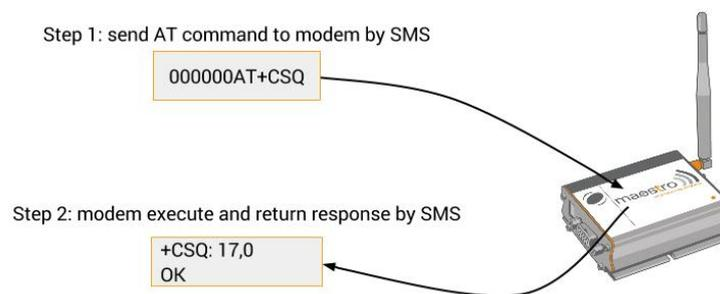
Figure 10.1.1: Example of remote AT command by SMS
