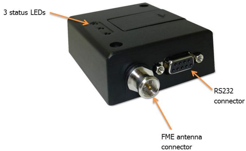
Figure 2: Connectors on front side of the Terminal
