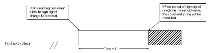
Figure 20.4.1: When T=1second the Command String #5 will be executed
