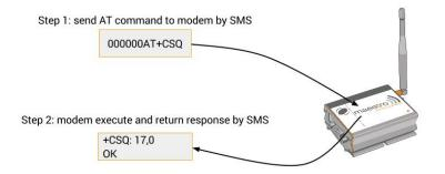
Figure 10.1.1: Example of remote AT command by SMS
