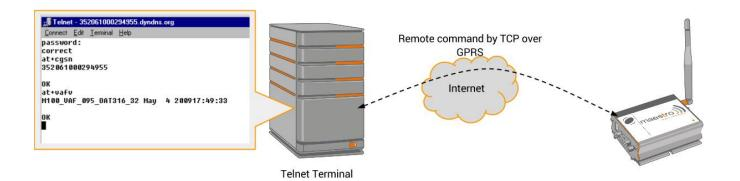
Figure 7.1.1: Example of TCP Terminal using Telnet
