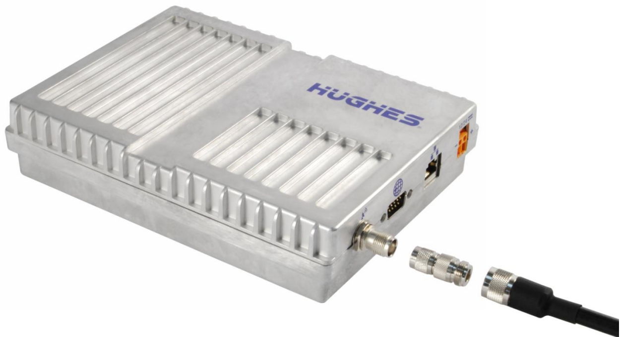
Figure 4-7 – Connect cable to TNC connector on IDU
