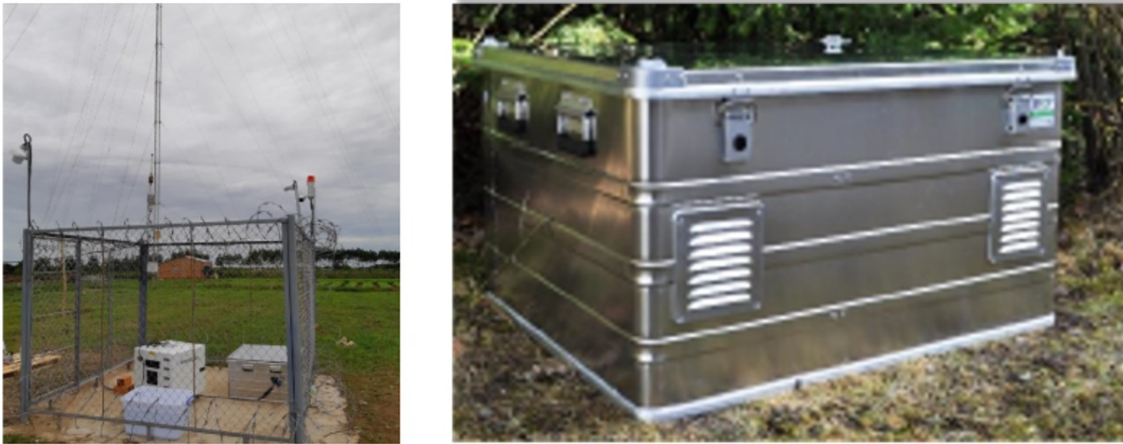
Figure 5 EFOY ProCube used to autonomously supply power to WindCube
