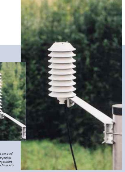
The new radiation shields are used in outdoor installations to protect relative humidity and temperature measurement instruments from rain and sun radiation.
