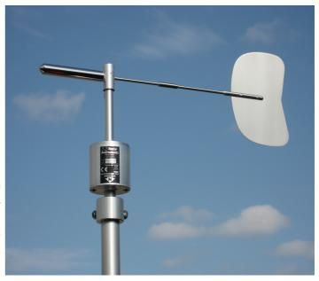
The 10K potentiometer means improved data-logger compatibility, and surge-protection is fitted as standard. Construction is from anodised aluminium alloys and stainless steels for exposed parts. Combined with the hard plastic (upper) plain bearing and precision ball races, the result is a robust instrument with a long service interval which is suitable for permanent exposure to the weather.
